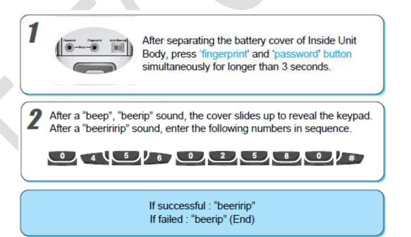
To check the completion of an initialization process, press the Cover Opening Button. Then a buzzer sound "beerip beerip beerip" will be heard.
